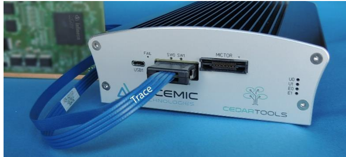
Figure 7: CEDARtools ® trace data online processing tool with high-speed serial trace connection to an Infineon AURIX™ processor
